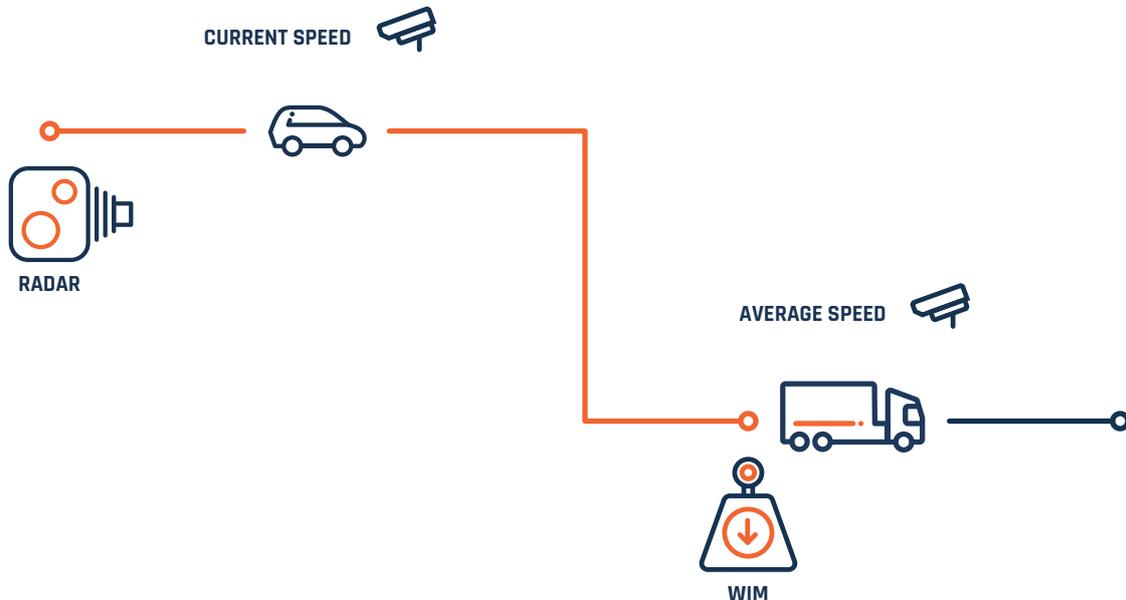
Section speed measurement can improve the WIM's performance as it is affected by driving fluency. Radars can be used at WIM sites to monitor the drivers' maneuvers. Knowing the changes in speed helps with validating the weight measurement.
